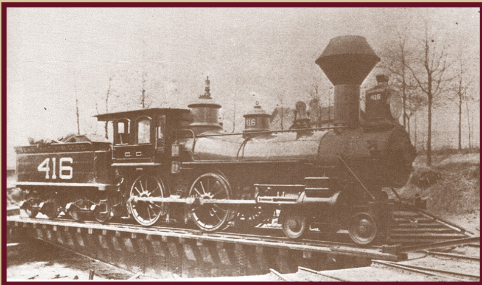
This steam engine was used on the Carolina Central Railway. SAL Number 416 was Carolina Central Number 26. Steam engines needed to stop for water approximately every 100 miles.
